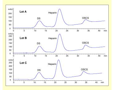
Column: Glycomix<sup>™</sup> SAX, 4.6 x 250 mm Mobile phase: A: 0.04% NaH<sub>2</sub>PO<sub>4</sub>, pH 3.0 B: 0.04% NaH<sub>2</sub>PO<sub>4</sub>+14% NaClO<sub>4</sub>, pH 3.0 Flow rate: 0.22 mL/min Gradient: 20% - 90% B in 60 minutes Wavelength: 202 nm Column temp: 25 °C 10 μL Injection volume: Pressures: 9.5 bar Sample: 20 mg/mL Heparin sodium 1 mg/mL Dermatan sulfate (DS) 1mg/mL Oversulfated chondroitin sulfate (OSCS) in H<sub>2</sub>O
