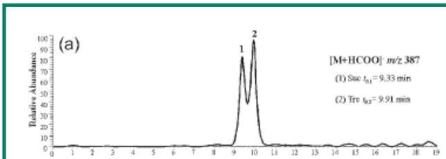
Figure 2: Separation of isomeric disaccharides Suc ( $t_r=9.33$  min) and Tre ( $t_r=9.91$  min) using ZIC®-HILIC column and gradient described in experimental.
