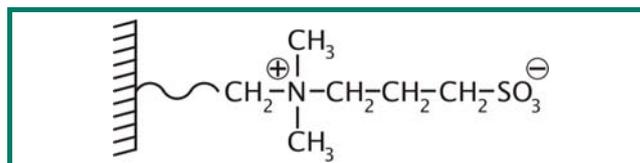
Figure 4: The Bonded Zwitterionic Sulfobetaine Group of ZIC®-HILIC.
